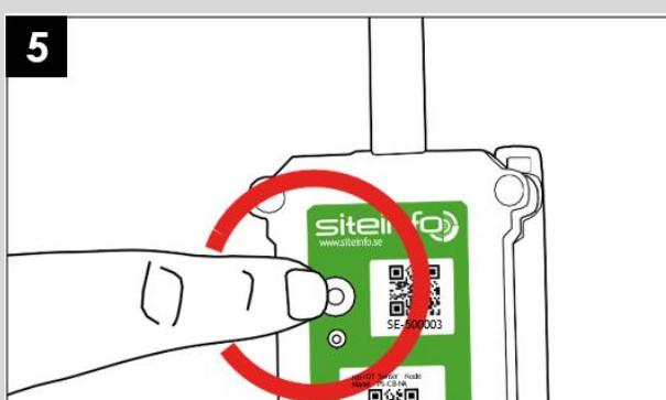
During Startup: Press the button until the LED flashes Green.
